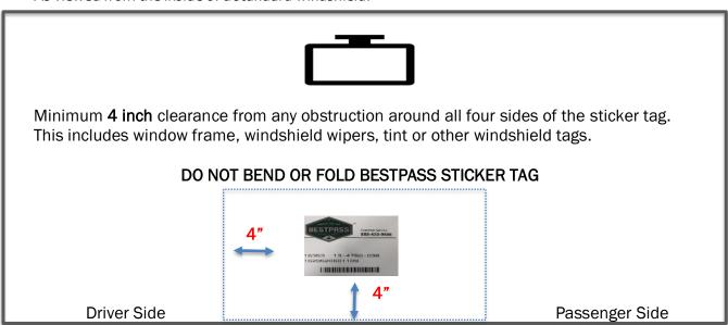
Once a sticker tag has been installed it cannot be removed or repositioned. Attempting to do so could result in the Bestpass sticker tag not functioning properly.
